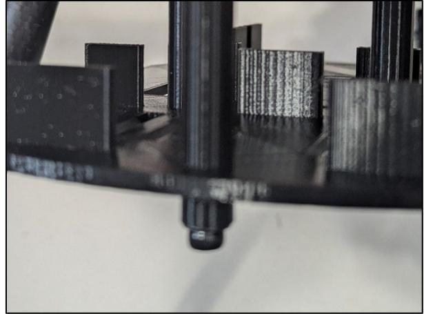
**Figure 49** Attaching spacer and Plate B
