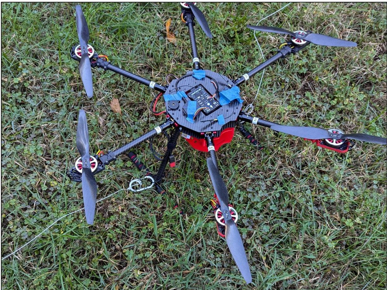
*Figure 73 The flight-ready UAV with flight controller, sensors, and propellers*
