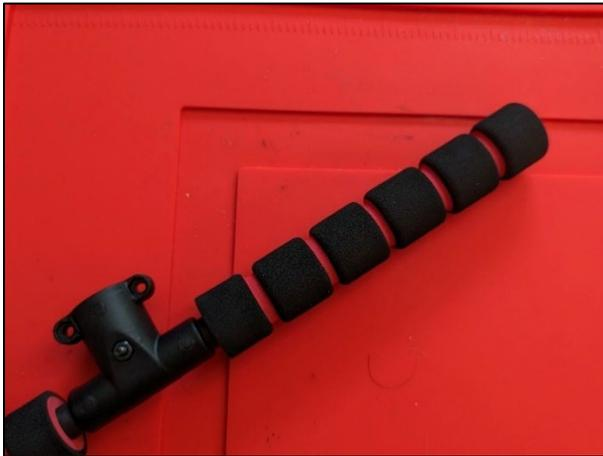
**Figure 31** Landing skid pad on narrow landing skid tube
