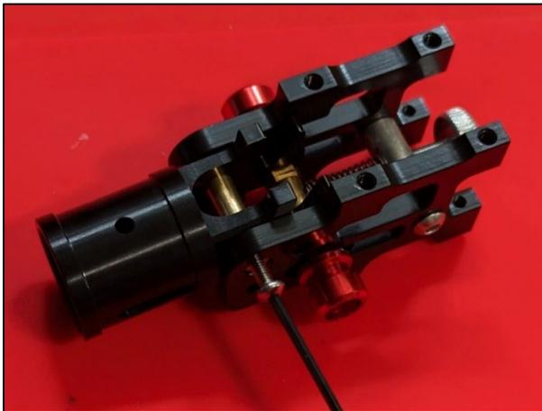
**Figure 19** Screw to remove from the locking hinge
