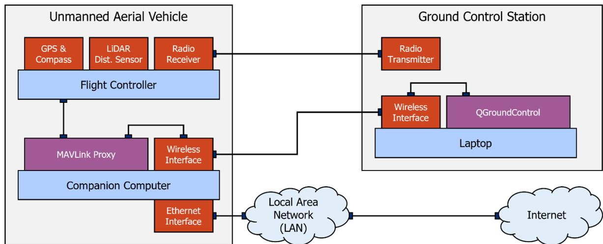
*Figure 1* A diagram showing the major components of the UAV and connected Ground Station
