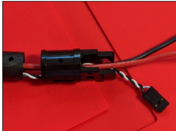
**Figure 20** ESC wires routed through the locking hinge
