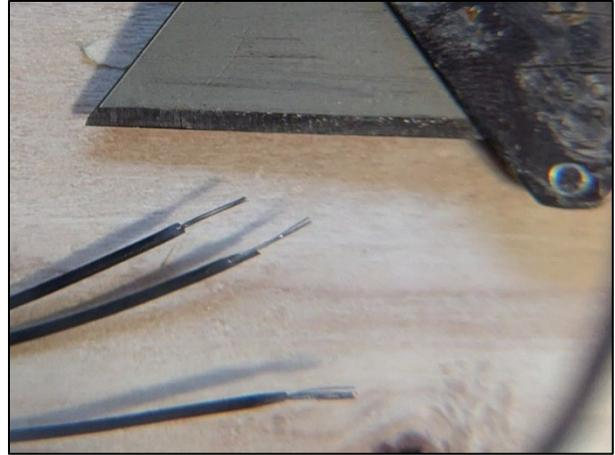
Figure 95 Insulation removed from wire with utility knife
