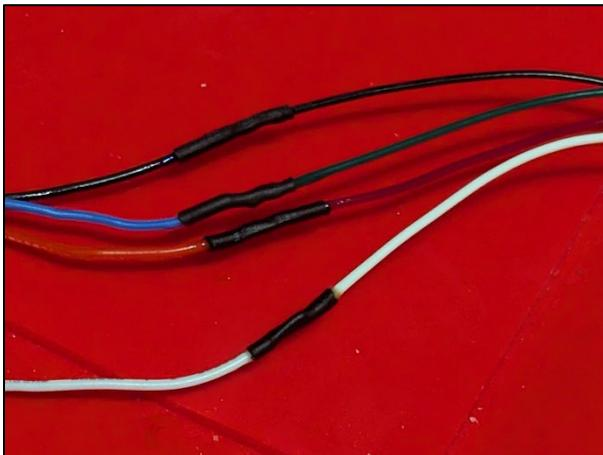
**Figure 127** Heat shrink tubing applied to individual wires
