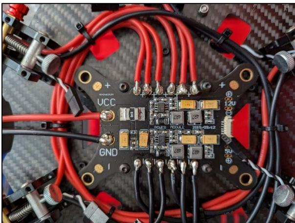
Figure 44 Excess wire secured neatly with zip ties
