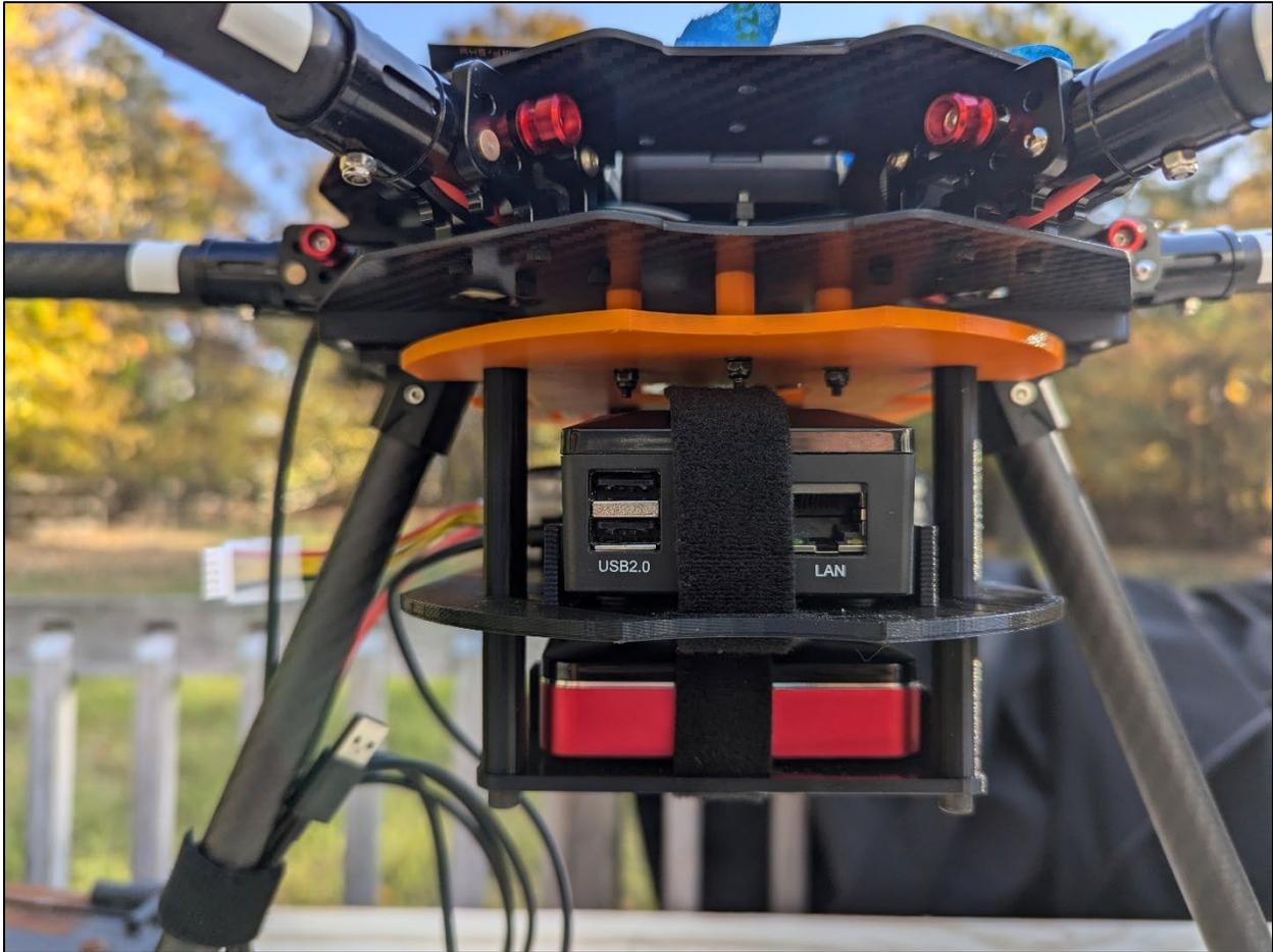
*Figure 111 The assembled UAV with attached companion computer*
