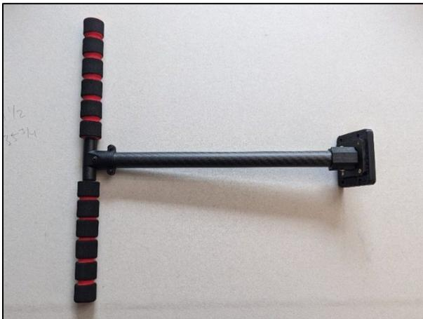
**Figure 33** Completed landing skid
