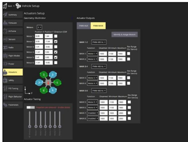
Figure 68 The Actuators page in 1.15(master) firmware
