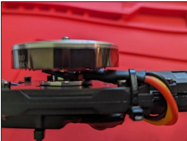
*Figure 17* Motor wiring zip-tied to the housing
