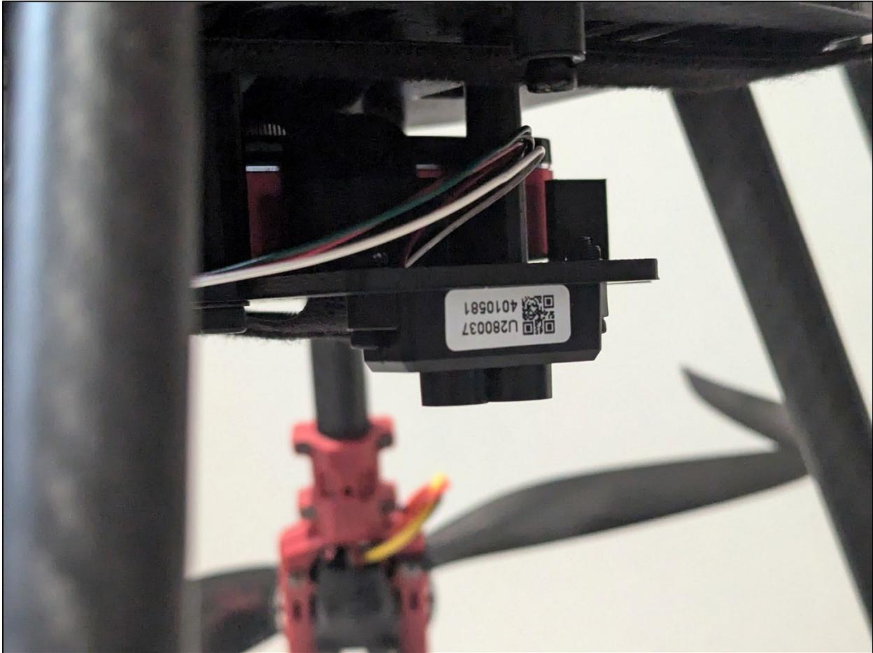
*Figure 137* Distance sensor mounted to the UAV frame
