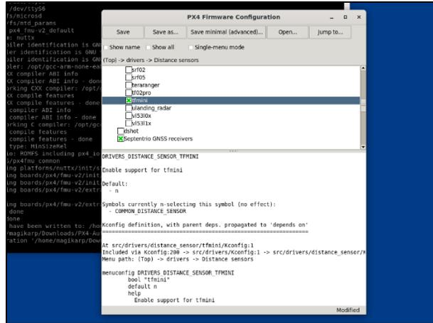
Figure 155 Checkbox enabling the tfmini driver
