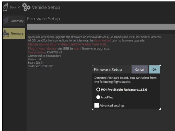
Figure 66 The Firmware Setup dialog box
