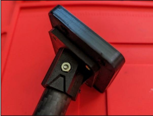
**Figure 29** Landing skid tube secured to mounting plate
