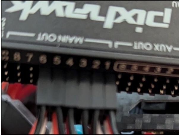
Figure 61 ESC cables attached to the flight controller
