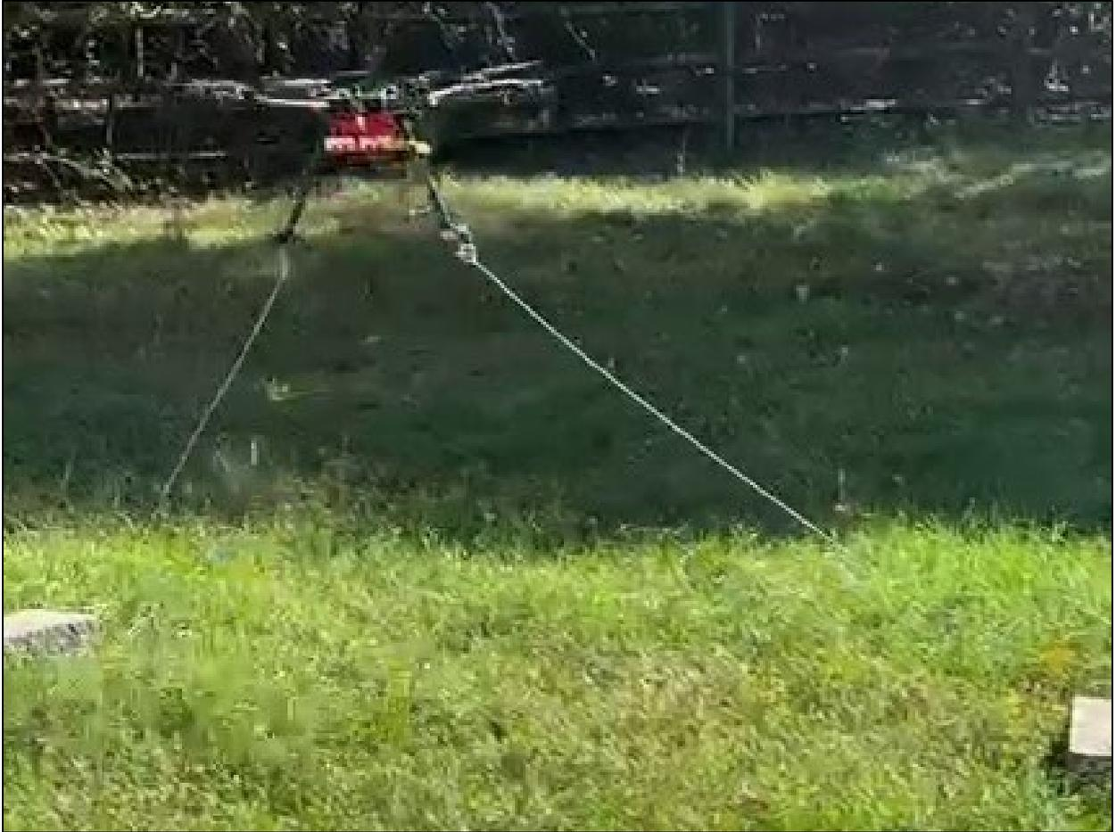
*Figure 78 Test flight with UAV tethered safely to the ground, allowed to hover a few feet in the air*
