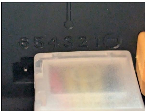
Figure 149 Correct alignment of balance port
