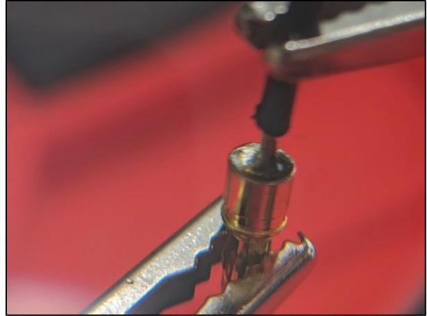
*Figure 5* Motor wire soldered to the male-end connector
