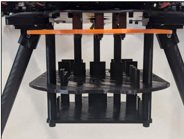
**Figure 52** The completed bottom extension frame
