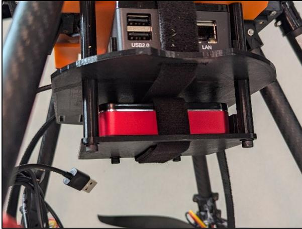
*Figure 140 Secondary battery secured*
