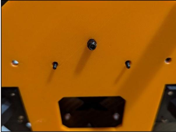
**Figure 48** Attaching Plate A to the UAV frame
