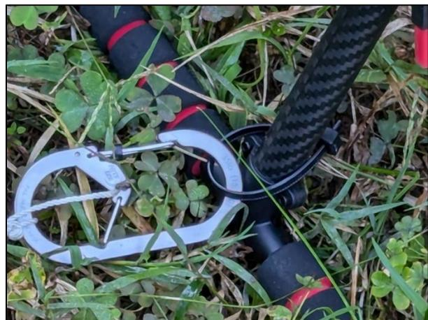
**Figure 75** Carabiner secured to UAV's landing skid
