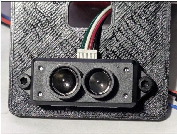
Figure 131 Distance sensor mounted with two bolts
