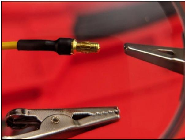
*Figure 6* Heat shrink tubing applied to connector
