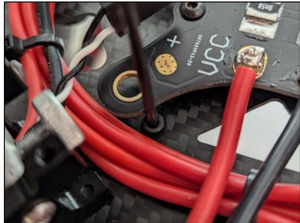
**Figure 47** Inserting the M2.5 bolt near the PDB's wing
