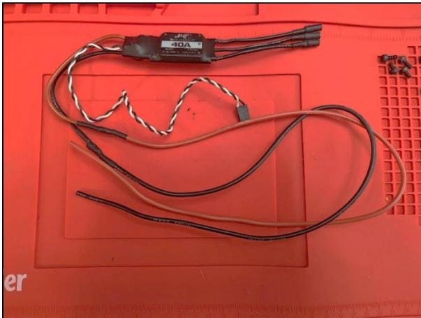
**Figure 10** The completed ESC assembly
