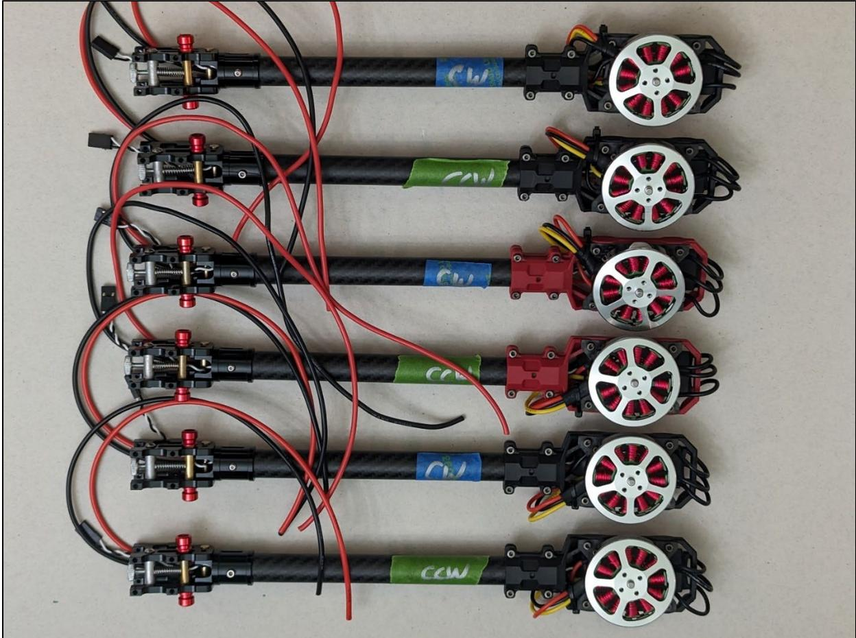
*Figure 26 The six completed arms with motors, ESCs, and locking hinges*
