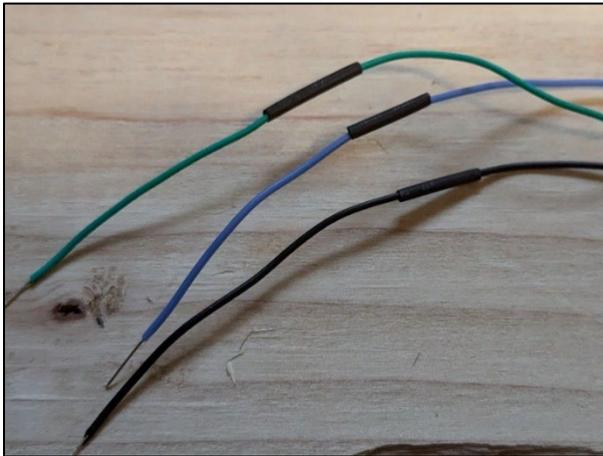
Figure 96 Stripped jumper wires with heat shrink
