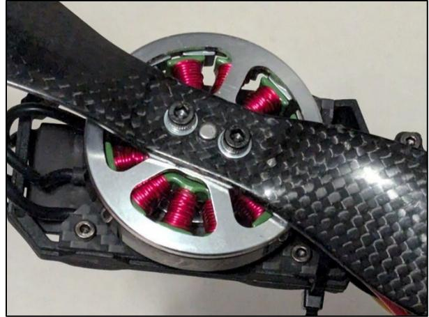
*Figure 72 Propeller installed on a motor*
