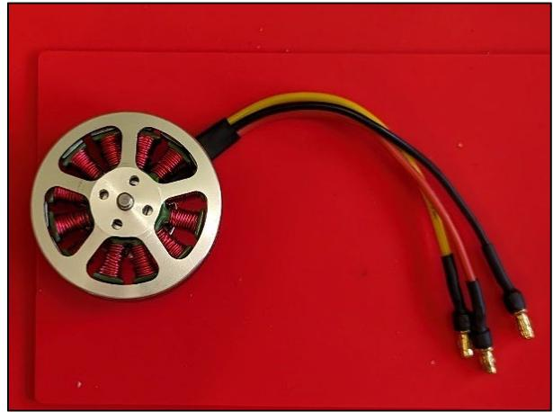
*Figure 7* The completed motor assembly
