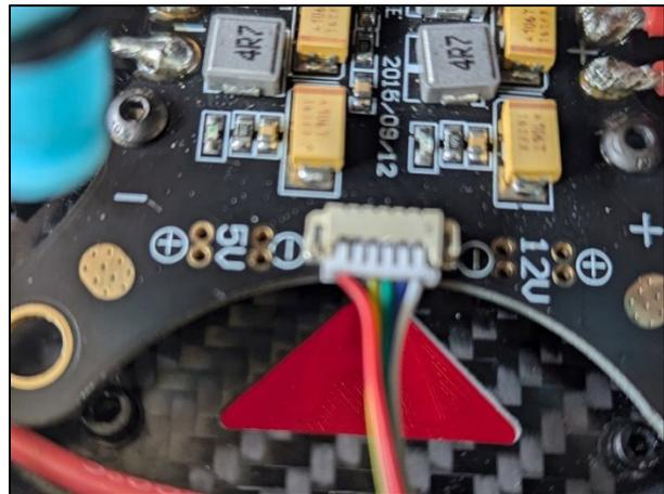
*Figure 54 Attaching flight controller power cable to PDB*
