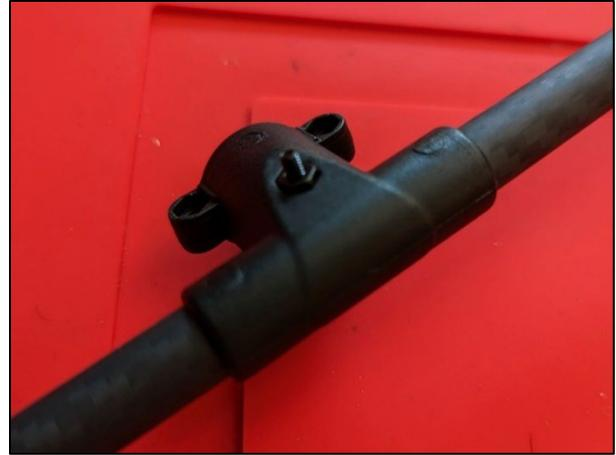
**Figure 30** Tee connector on narrow landing skid tube
