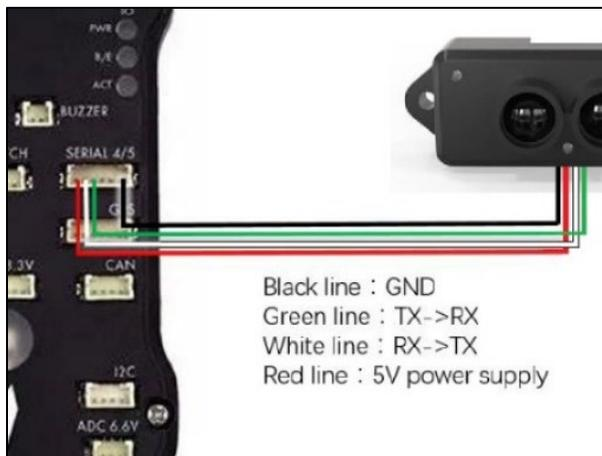
**Figure 121** TFmini wiring diagram from Ardupilot
