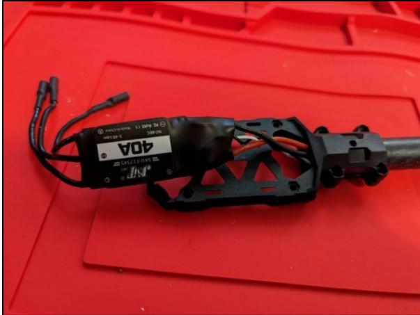
*Figure 13* ESC wires fed through the housing and arm
