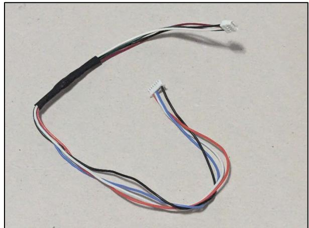
**Figure 128** Heat shrink tubing applied to all wires
