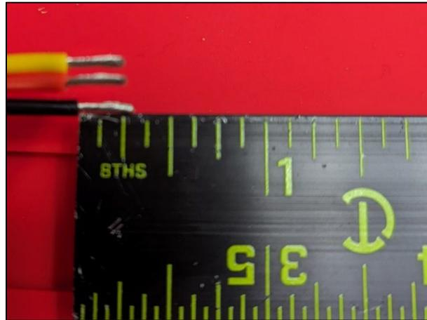
*Figure 3* Ends of stripped motor wires
