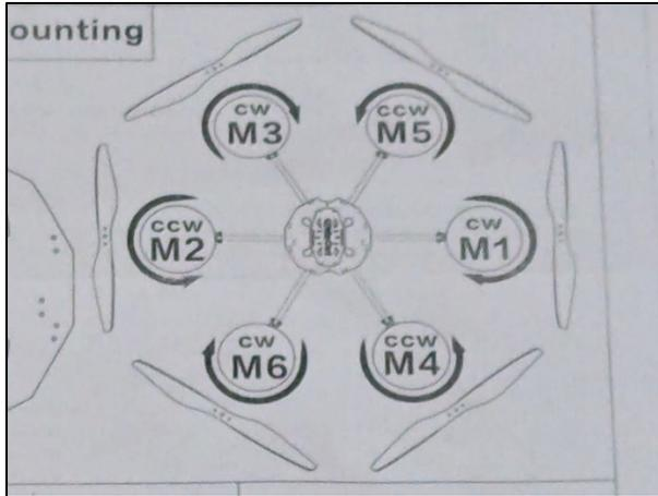
*Figure 71 Correct propeller orientation*
