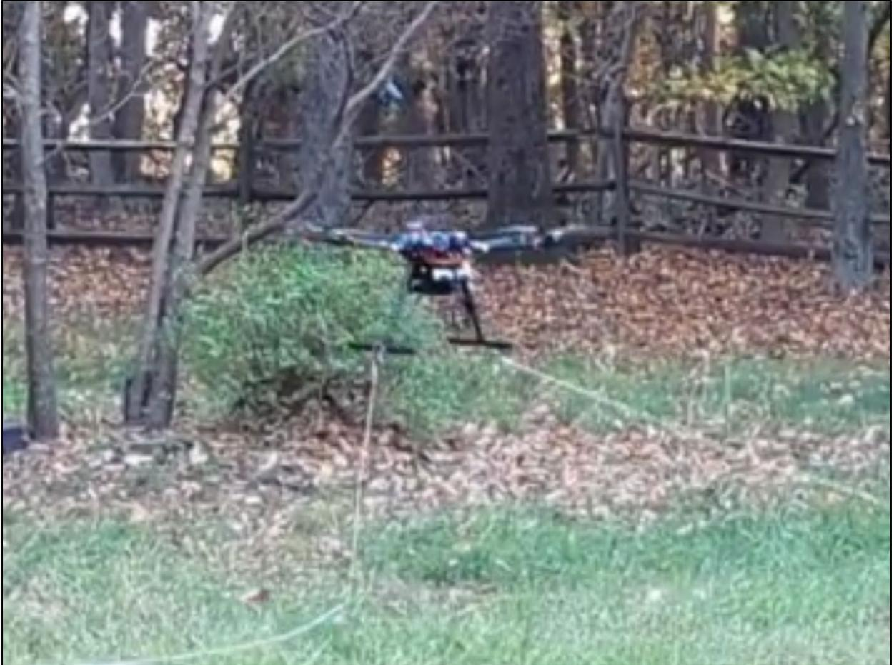
*Figure 120* Test flight with UAV tethered safely to the ground, executing takeoff mission from QGroundControl
