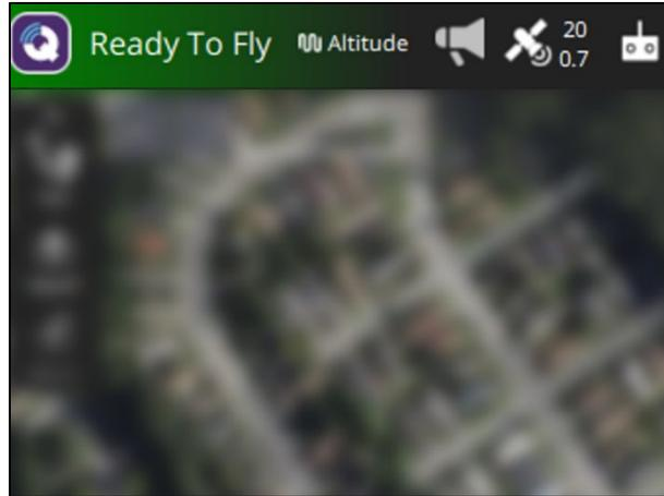
Figure 70 "Ready to Fly" with no pre-flight alerts
