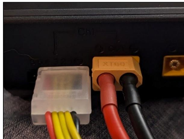
Figure 148 Balance port and XT60 cable connected
