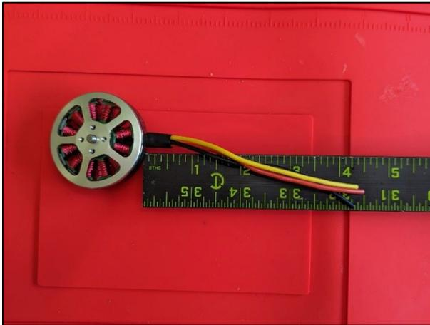
*Figure 2* Motor with wires cut to approximately  $4\frac{1}{2}$  inches
