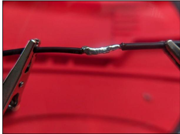
**Figure 9** ESC wire and extension soldered together
