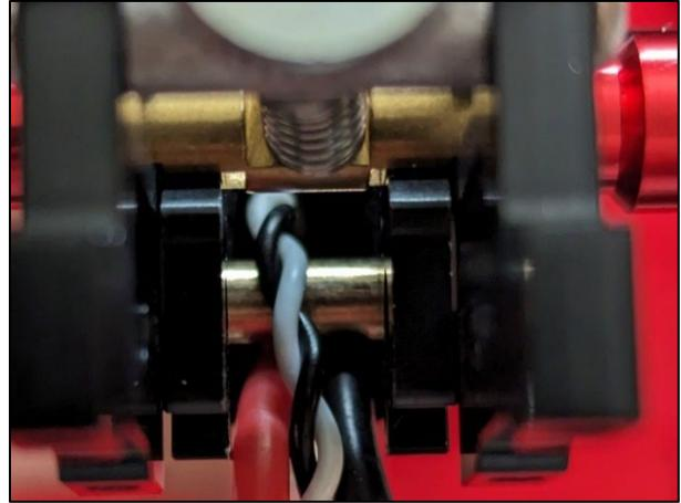
*Figure 22* ESC wires routed around the barrel nut
