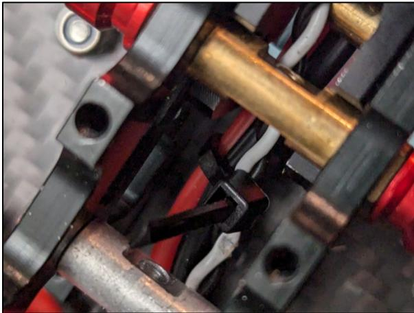
*Figure 23* ESC wire bundle secured with a zip tie
