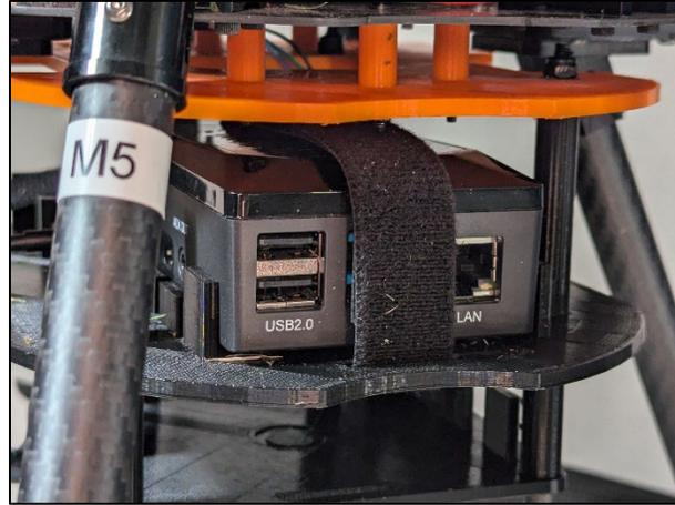
*Figure 108* Companion computer secured to the frame
