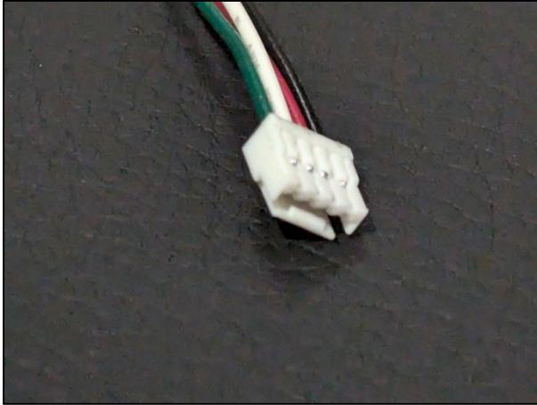
**Figure 123** Connector for the distance sensor
