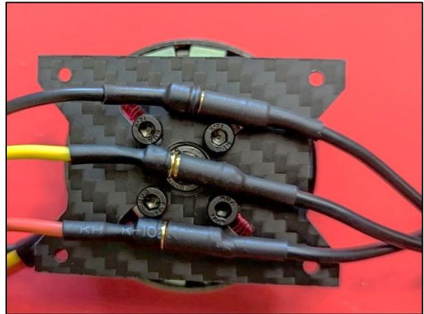
*Figure 16* Example routing of wires around bolt heads
