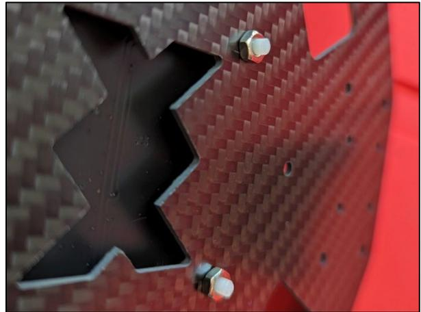
**Figure 39** Spacer bolt secured to bottom plate with nut
