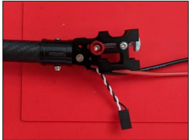
*Figure 24* Hinge locked in the "up" position
