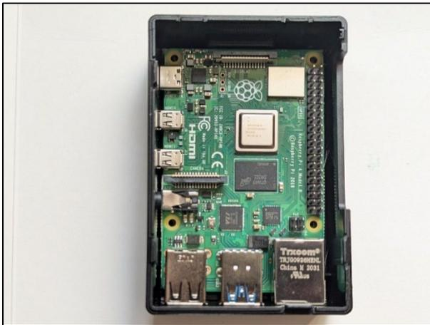
*Figure 89* Raspberry Pi installed in case
