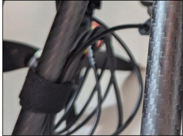
*Figure 141 Excess cable secured*
