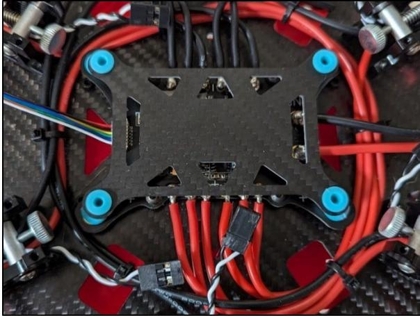
*Figure 57 Completed flight controller mounting plate*
