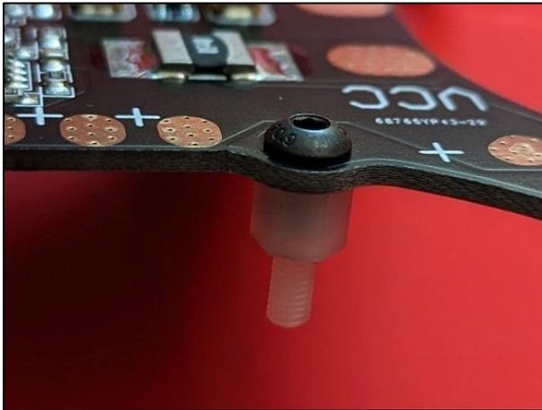
**Figure 38** Spacer bolt secured to power distribution board
