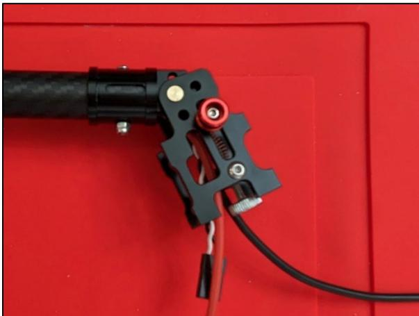
*Figure 25* Hinge locked in the "down" position
