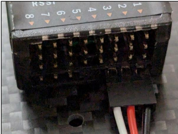
**Figure 59** Cable connected to receiver's SBUS pins
