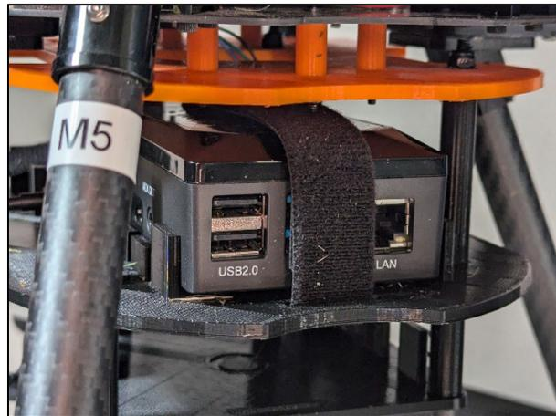
*Figure 139 Companion computer secured*
