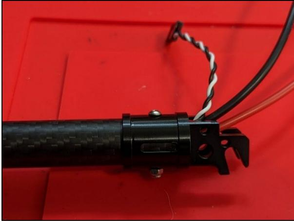
*Figure 21* Small hinge piece secured to the arm tube
