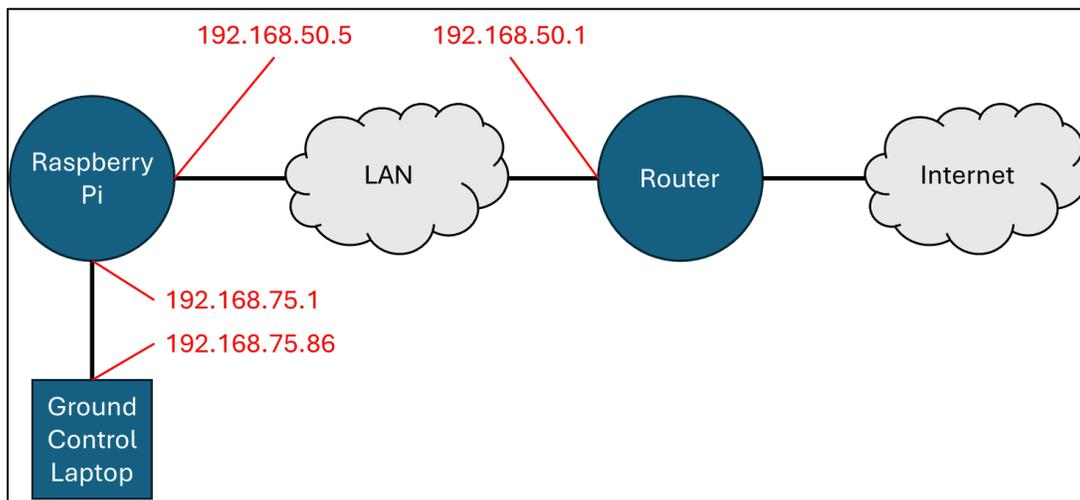
Figure 104 A network diagram showing the companion computer's IP connections to other devices.
