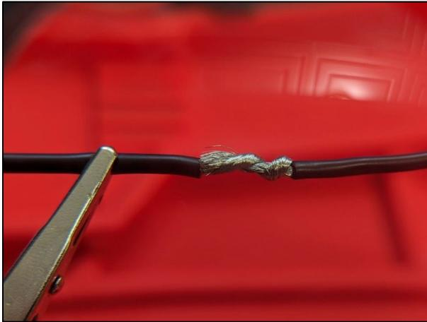
**Figure 8** Additional wire twisted around the ESC wire
