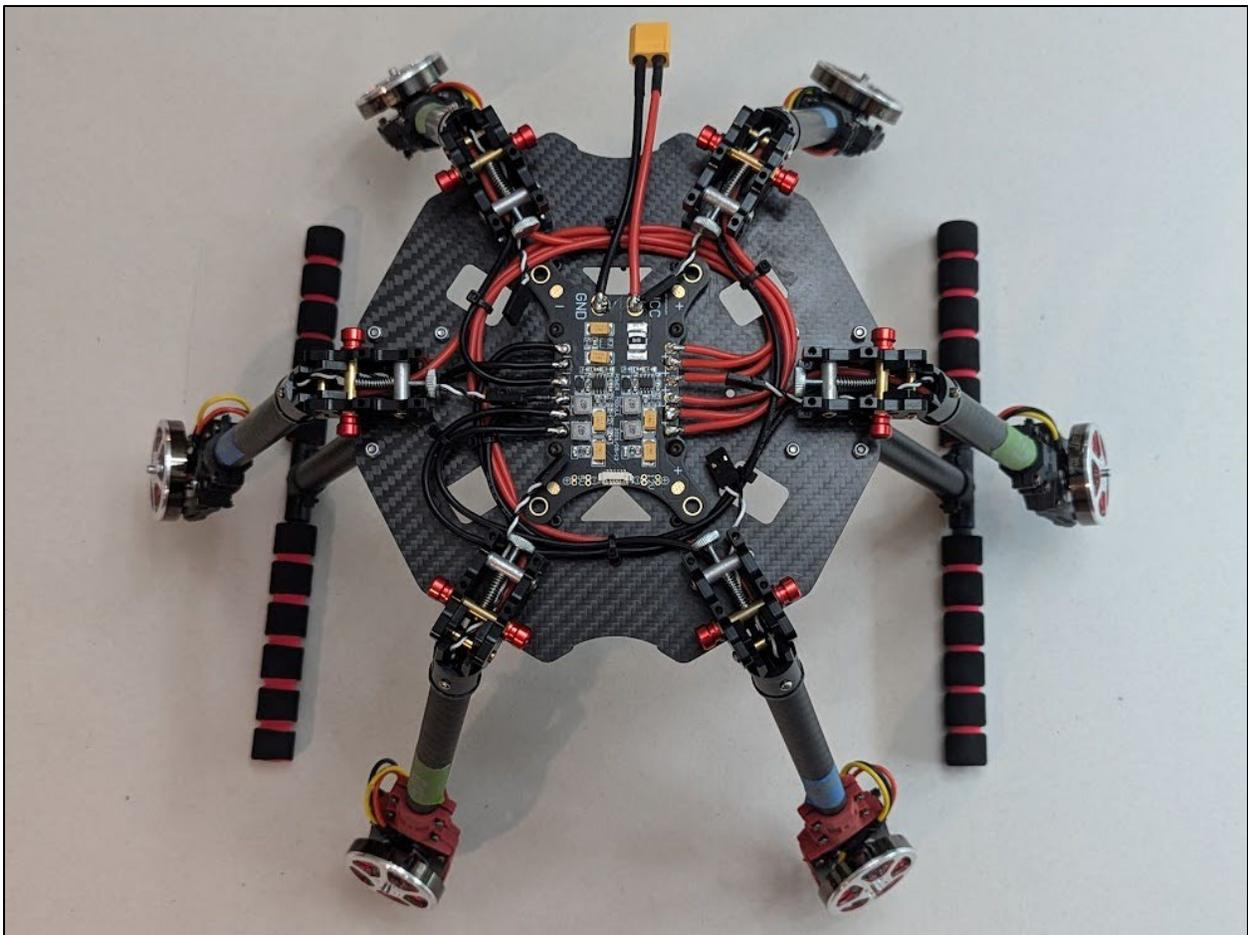
*Figure 45* The UAV frame with arms, landing skids, and power distribution components attached
