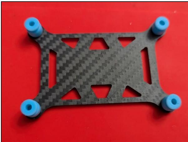
*Figure 53 Spacers attached to mounting plate*
