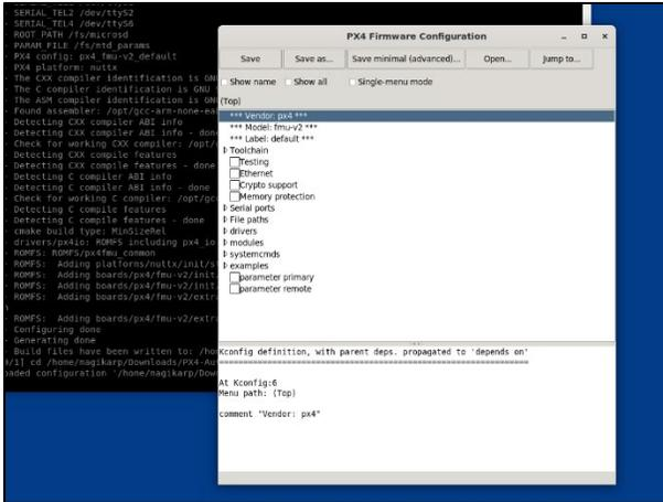
Figure 154 PX4 Firmware Configuration GUI
