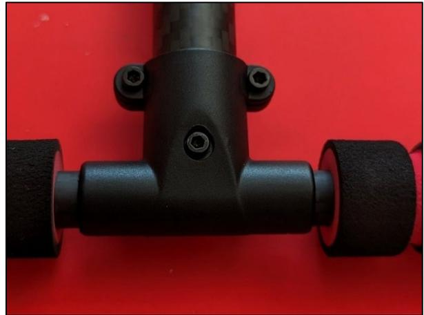
**Figure 32** Landing skid secured to wide landing skid tube
