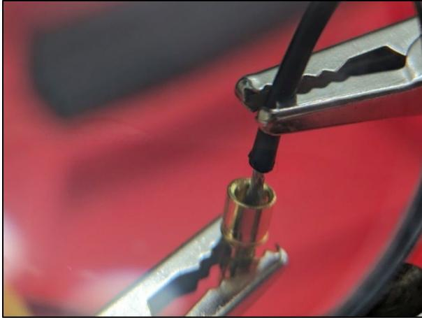
*Figure 4* Motor wire centered in the male-end connector
