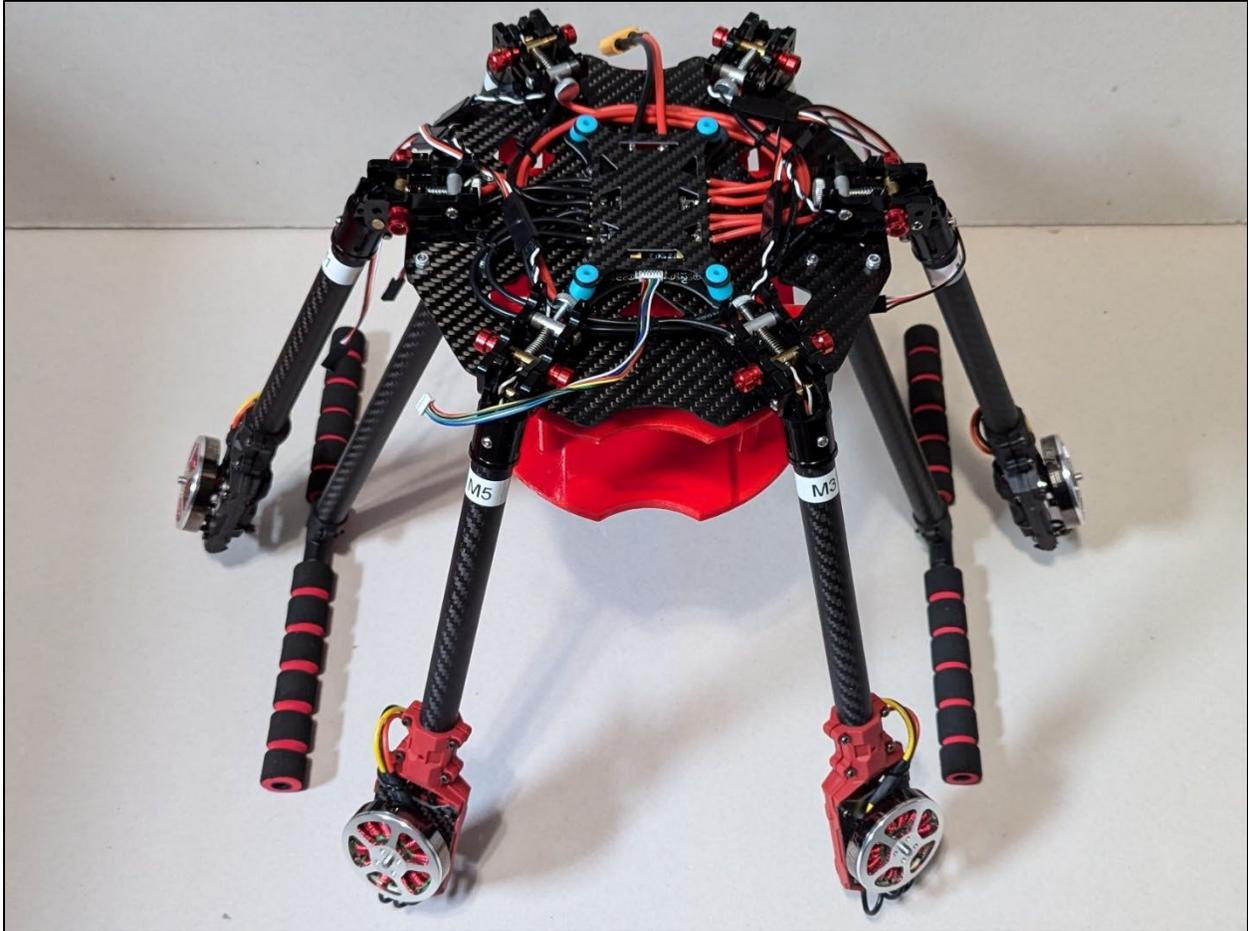
*Figure 58 The UAV with completed bottom attachment points and flight controller mounting plate*
