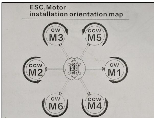
**Figure 11** ESC, Motor Installation Orientation Map
