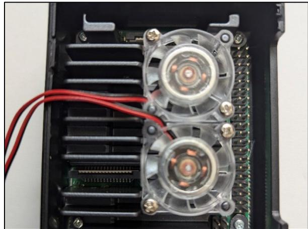
*Figure 90* Fan installed on top of Raspberry Pi
