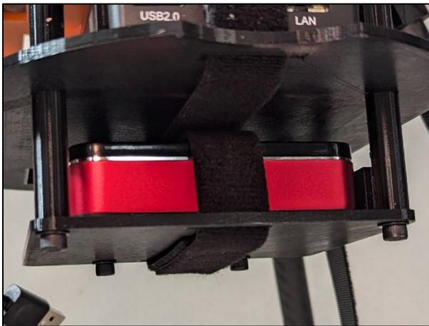
*Figure 109* Secondary battery secured to the frame
