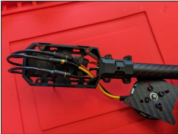
*Figure 15* Motor wires connected in the housing
