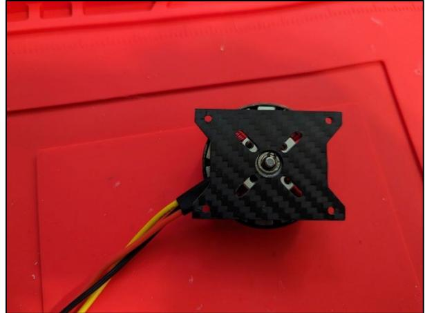
*Figure 14* Motor attached to motor mounting plate
