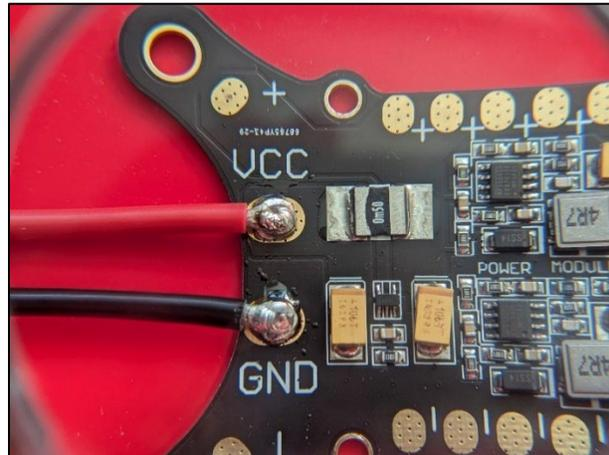
*Figure 35 Power cable soldered to PDB*
