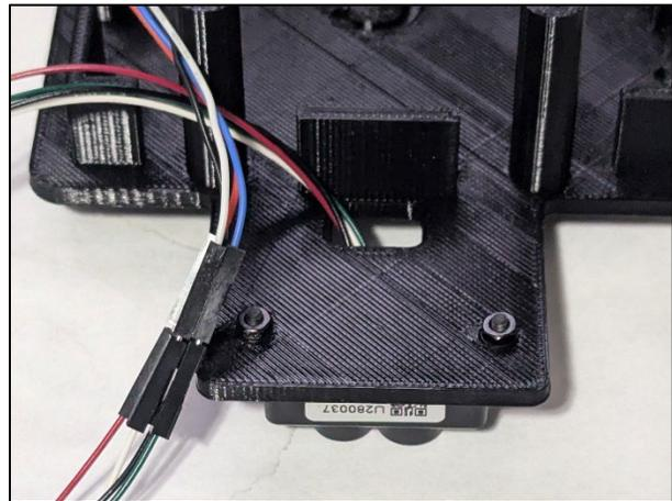
Figure 132 Correct orientation of the distance sensor
