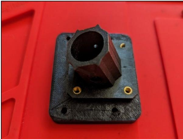
*Figure 27 Mounting plate on mounting block*
